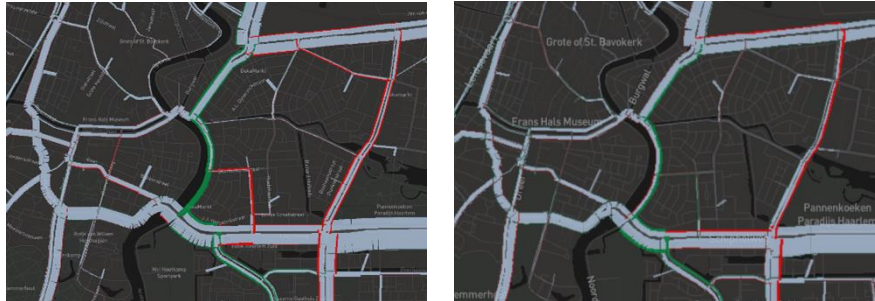
Figure 3.8: Difference plot of traffic intensities between Hub North (left) and Hub Tunnel (right) compared to the reference 2030 scenario, based on the infrastructure configurations as presented in Figure 3.1 and Figure 3.3. Red indicates an increase in the number of cars, green a decrease. For example, more people use the Slachthuisstraat, a possibly undesired effect.
